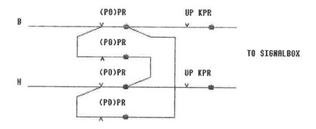
When the barriers are raised the UP KPR (barriers up indication repeat relay) is energised.
