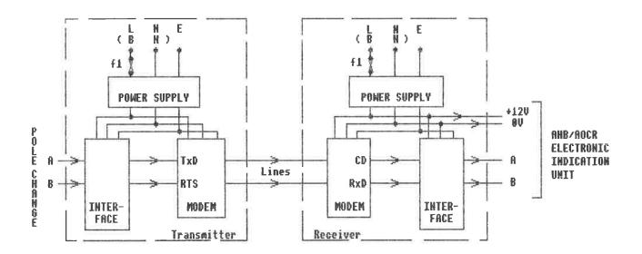
The transmission system is designed to work in conjunction with the A.O.C.R. Electronic indication unit and allows operation over British Telecoms lines.
