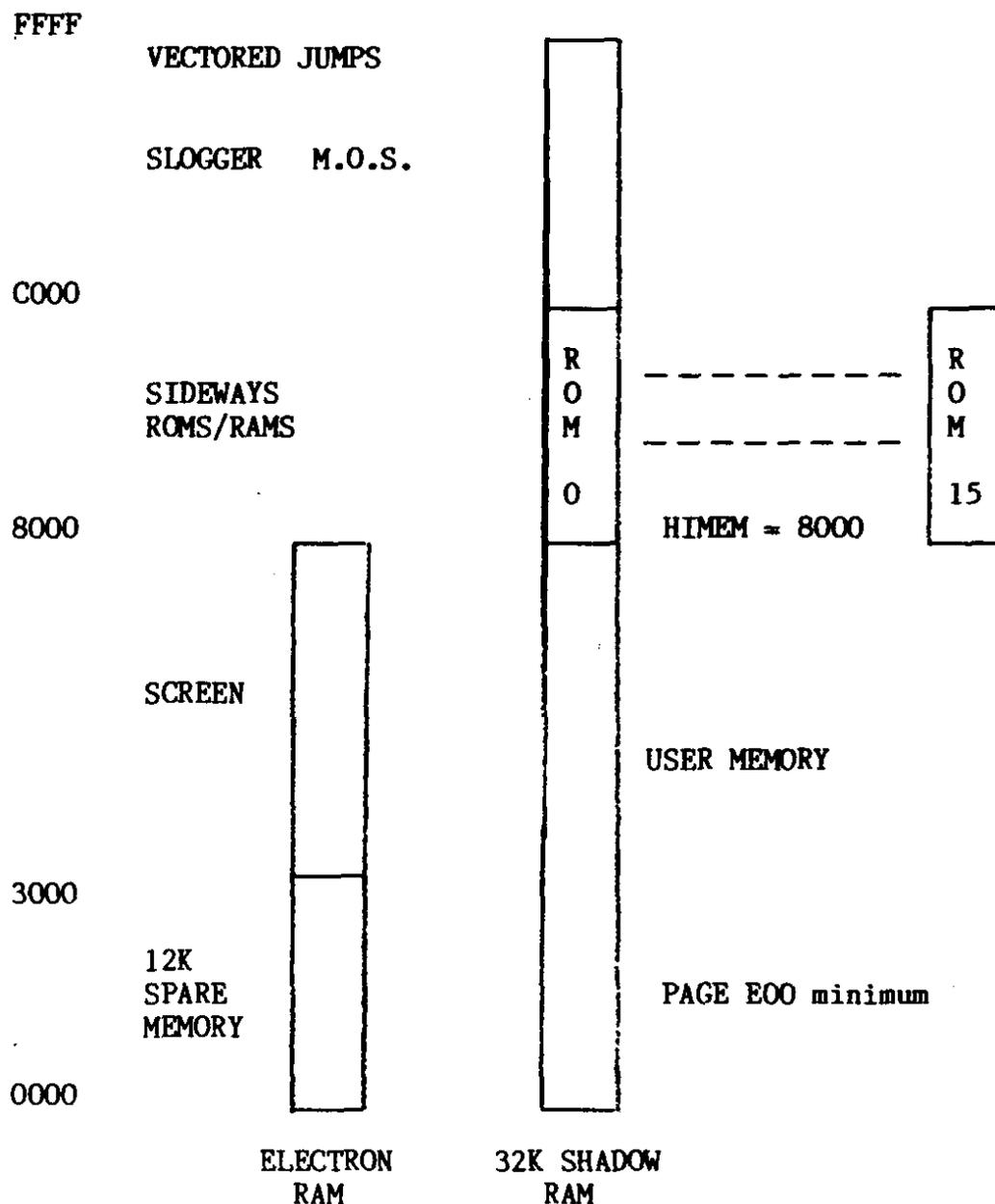
With the Electron running in Shadow mode the Electron RAM, including screen, is pushed to one side and is totally replaced by the fast 32K RAM. All programs, either BASIC, machine code or any other language may use memory through to 8000 with no interference from the screen.
