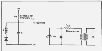
Fig. 11 (left) A simple HF oscillator circuit using a tunnel diode and Fig. 12 (right), driving an LED from an AC supply.
