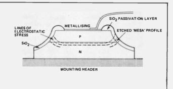
Fig. 4 The sides of a high voltage rectifier chip are etched away at an angle to deflect electrostatic stress away from the edge of the junction.
