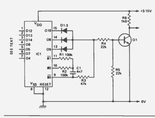
NOTE: IC1 = 4060 OI = 2N3904 OR EOUIVALENT D1.3 = 1N4148 (SEE TEXT) R1.2,C1 CORRESPOND TO BASIC FREQUENCY OF ABOUT 1HHz OUTPUT IN THIS CONFIGURATION CONSISTS OF GROUPS OF 128 PULSES INTERSPERSED BY GROUPS OF 896 "MISSING" PULSES TRANSISTOR STAGE INVERTS
