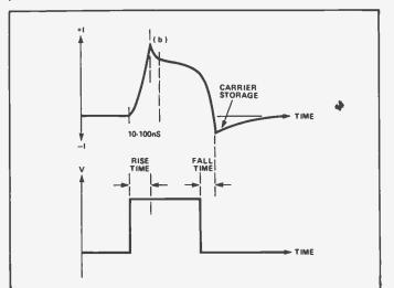
Fig. 7 Carrier storage following a reversal of the applied voltage in a PN junction diode.
