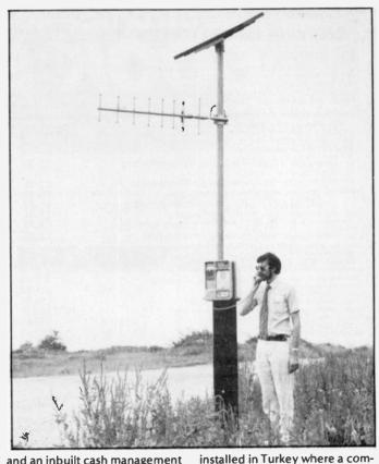
and an inbuilt cash management system reports when the coin box is 75 per cent full. For simple installation a metal plate at the foot of the payphone pole is dropped into a concrete base.
