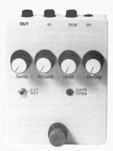
triggering method is used, the attack, hold, and decay controls still function. Because the envelope shape is completely adjustable and the unit can be controlled by a variety of inputs, it can be used as an envelope shaper in its own right.
