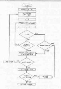
Fig. 1 Flowchart for 27256 programming routine.
