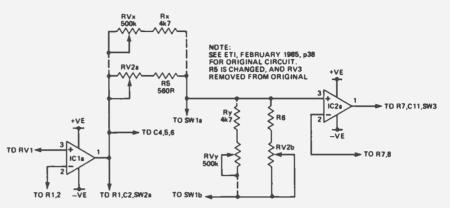
attached by dashed lines. A 500k linear dual pot (designated RVa, b) in series with 4k7 resistors (to prevent too low a minimum resistance) is wired across notch frequency control RV2a, b and associated resistors R5 and R6.
