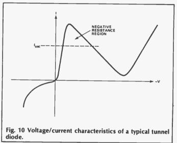
At very low reverse bias levels, the thermal energy of the electrons in the semiconductor is high enough for them to 'tunnel' through this depletion layer, and the junction conducts. However, as the reverse voltage is increased the thickness of the depletion layer increases, so the tunneling effect, even with an increased potential difference, begins to lose ground. The current then begins to fall as the potential is increased, giving what is known as a negative resistance characteristic.
