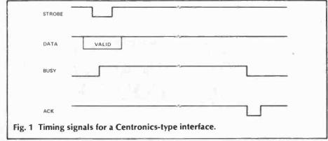
(printer) responds by pulling the BUSY line high for as long as is necessary to process the data received. The BUSY line is then pulled back low and a short 'active low' pulse is output on the ACK line to indicate that the transfer is complete and the next. data byte may be transmitted. The busy period may be anything up to one second during carriage return on a slow printer, and the transmitting computer is normally idle during this time.
