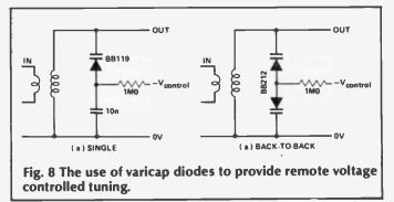
voltage across it. Such a diode appears to consist of two conducting regions separated by the depletion layer between them, which acts as a dielectric. Typical devices have capacitance values in the range 3-50pF, depending on device and applied voltage.
