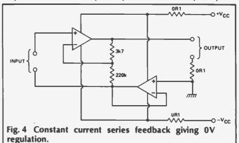
$\frac{1}{2}$ x5532 in unity gain configuration this is 10 milli ohms, rising to 30 milli ohms at 20 kHz). Also, the increase of current in the stage output is complemented by a reduction in the 0V regulator - which means that while the amplifier is operating in Class A mode (about 99% of the time), overall current consumption is constant.
