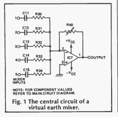
No VU metering system has been provided since it is assumed that the recorder used will have this facility.
