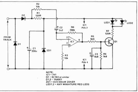
form a potential divider which holds Q1 just off under these conditions and C3 removes most of the AC. When the voltage across the track drops and the car slows down, the output of the IC rises to around 4V increase sound output.
