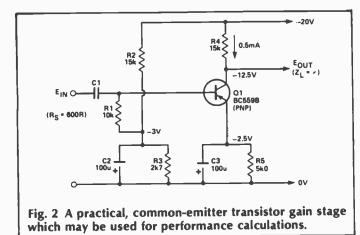
Unlike valves and FETs, transistors have a DC conductive path between their three connections, so the output impedance is influenced by the input circuit impedance and vice-versa, and all of these including the current gain, are influenced by the operating current of the device.
