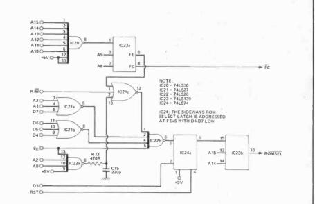
Fig. 4 Suggested interface circuit to link basic Electron and the second processor.
