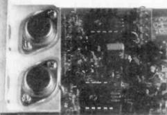
All of these modules now incorporate the following: • HP Protection — Automatic shutdown to prevent damage from unstable signal source.
