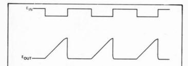
Fig. 5 Slew rate limiting caused by stray capacitance on a constant current source load.
