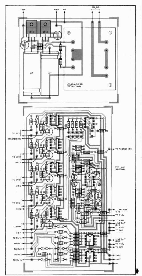
RV6, with a master fader, RV10, controlling their overall level so that it can be faded down if, for example, a voice-over commentary is to be superimposed from the master mic.
