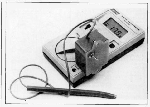
to 10mV per °C. Low power semiconductors are used making the quiescent current drain of the Heat Pen less than 1mA.
