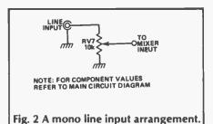
having outputs conforming to the DIN standard — in which the output is arranged to provide 1mV for each 1K of load impedancy the alternative arrangement of Fig.
