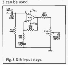
This is quite a versatile system, and can be used with any input source where a flat frequency response is all that is needed, and where the input signal level will not exceed more than about 0.5V RMS.
