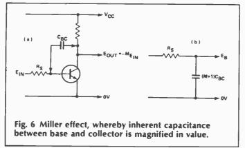
Supposing, therefore, that the stage gain is 150x, and the base-collector capacitance is 5pF, the actual capacitance seen at the transistor end of the source resistor is  $5 \times 150$  pF = 750 pF, which will have a considerable effect on the HF response of the circuit.
