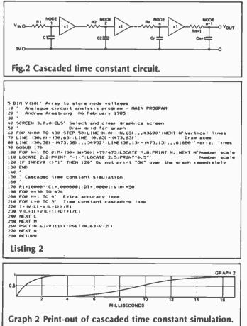
result will look like Graph 2 in which a single RC time constant is shown for comparison. In this graph, it is assumed that the current drawn from each RC stage by the succeeding one is negligible, or that they are separated by voltage followers, as in Fig. 2. The effect of ten cascaded time constants is plotted. The routine used is shown in Listing 2.
