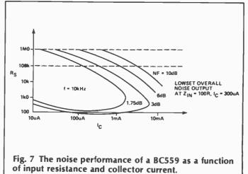
Happily, improvements in device manufacture have led to better characteristics, so, if you have a choice, use a device with a high 2N or BC number, rather than a low one. A BC549 is likely to be a better device, at the same cost, than a BC109, since these are both of the same type, only differing in date of design. Surprisingly, PNP small signal devices are better than NPN in this respect because the current flow in the base region — which is of N type — is due to electrons rather than holes.
