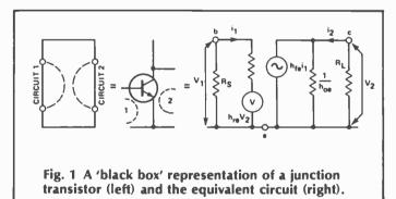
However, in addition to these we have the transfer characteristics, such as the forward current transfer ratio. This is written as hF if we are talking about DC values (usually referred to as static conditions) or hf if we are referring to dynamic (AC) characteristics. The reverse, or feedback parameter, h12, becomes h.
