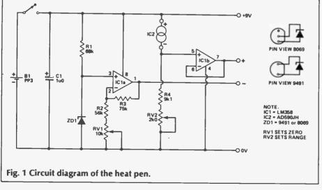
mly fitted at the ¾" pitch. The PCB, along with a PP3 battery fits neatly into a smart plastic potting box. The probe is mounted in a ball point pen casing and is connected to the PCB via a screened cable.
